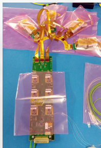
Disassembled PLT quadrant spare
