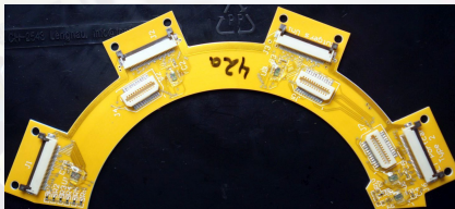
PLT port card (left) and LCDS chip (right)
