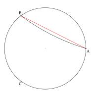
of them fit along that line than along the one that appears curved to us. If they do the same between B and C, and between C and A, and measure the angles, they will find the sum of the angles of their triangle is less than  $180^{\circ}$ ! Geometry is not Euclidian or Lorentz when observed in an accelerating coordinate system.
