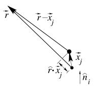
$$\frac{d\sigma}{d\Omega} = \frac{k^4}{(4\pi\epsilon_0 E_i)^2} \left| \sum_j \left[ \vec{\epsilon}^* \cdot \vec{p}_j + (\hat{r} \times \vec{\epsilon}^*) \cdot \vec{m}_j / c \right] e^{i\vec{q}\cdot\vec{x}_j} \right|^2.$$
