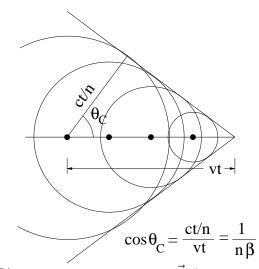
Note that the radiation is 100% polarized because the  $\vec{E}$  field is in the plane including the charged particle's trajectory, while  $\vec{B}$  is normal to that plane.
