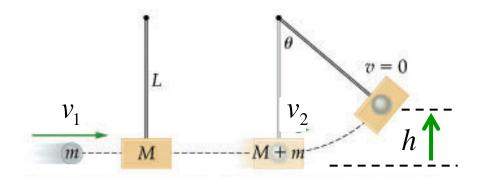
A bullet  $(m_a, v_1)$  is fired into clip of pendulum which swings to height h. What is  $v_1$ ?
