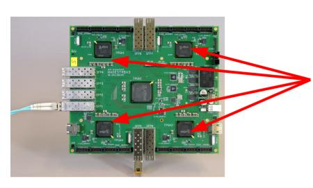
Each peripheral FPGA manages 1 interface board Each interface board manages 4 PADIWAS
