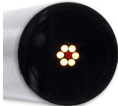
3. Adjust the height of the optical probe. The distance of a few mm between the probe and the sample gives an optimal signal.
