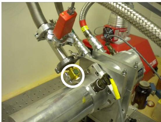
**11.** Close the pumping valve (marked in the picture above, shown as open). This is to prevent a sudden rush-out flow of air when the pump starts. Such a flow may ruin the wiring of your sample.
