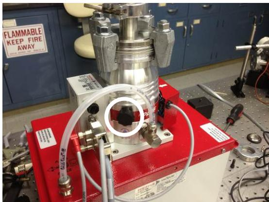
**12.** Make sure the venting valve on the back side of the pumping station is closed (marked in the picture above).
