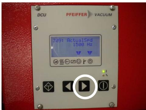
**13.** Turn on the pumping station power. Select parameter 309 by pressing the right pointing triangle soft button on the control panel (see picture above). This parameter gives the actual rotation speed of the turbo pump and should be 1,500 Hz during normal operation.
