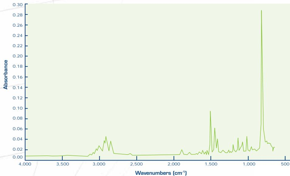
Figure 6. FTIR Absorbance Spectrum of Parylene C
