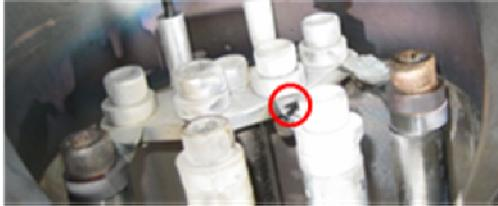
6] Inspect the inner surface of the cap. If there is a considerable accumulation of thick silver film, it may cause shorts in the circuitry of the chamber. Remove the deposit by scratching it off with a sharp clean tool, such as tweezers, knife or a screw driver. After this, put the cap back on and fix it with the two nuts (while tightening the nuts it is important to press on the cap down between the posts to prevent cap tilting which may cause a short).
