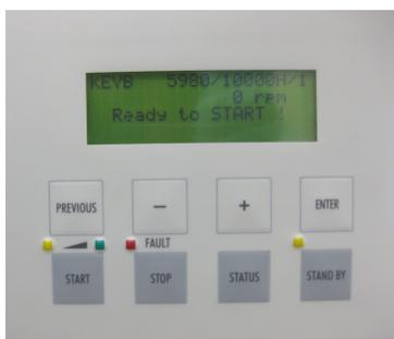
12] Press "start" button; the controller will display "start delay" (1 minute) and then will accelerate the turbo pump; wait until speed reaches 27000 rpm. When the pressure reaches sub mTorr range, turn off the vacuum gauge to avoid damaging organic samples with a gauge effect (this is not necessary for devices coated with parylene).
