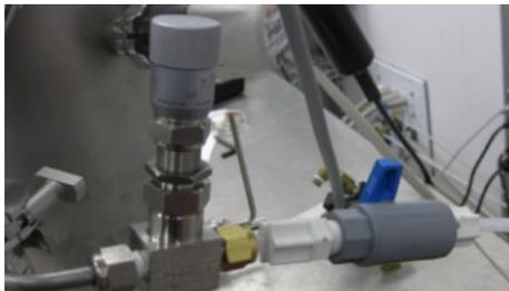
10] Wait for the pressure to drop to about  $10^{-2}$  Torr, and then hand tighten the lower door knobs again.
