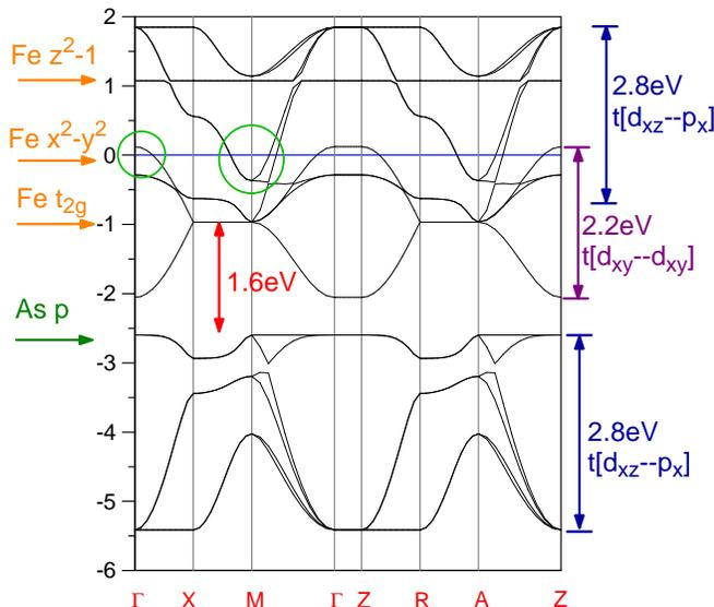
FIG. 1: (Color online) Tight-binding the band structure of LaFeAsO. The circles at the Fermi level on the  $\Gamma$  and  $M$  points indicate the hole and electron pockets, respectively.
