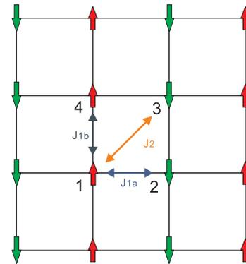
FIG. 2: (Color online) Spin arrangement and exchange interactions in the Fe plane of the striped  $Q_m$ -AFM phase. The arrows on lattice sites indicate the Fe spin directions. The double arrows indicate the nearest neighbor AFM interaction ( $J_{1a}$ ), FM interaction ( $J_{1b}$ ) and next nearest neighbor AFM interaction ( $J_2$ ).
