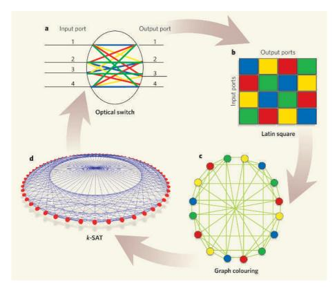
Figure 2 | Finding satisfaction. Constraint-satisfaction problems form a large class of practical computational problems, and encompass well-studied special cases such as the graph-colouring and *k*-SAT problems. a, An optical switch. The task is to assign a wavelength of light to each input–output path, such that a given wavelength is not assigned more than once to any input or output port.
