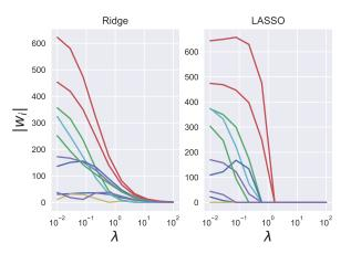
FIG. 15 Regularization parameter  $\lambda$  affects the weights (features) we learned in both Ridge regression (left) and LASSO regression (right) on the Diabetes dataset. Curves with different colors correspond to different  $w_i$ 's (features). Notice LASSO, unlike Ridge, sets feature weights to zero leading to sparsity. See Notebook 3.
