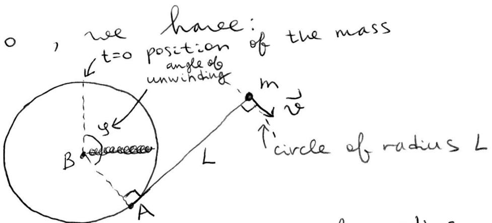
The mass is on a circle of radius  $L$  & the velocity  $\vec{v}$  is tangential to the circle, with  $|\vec{v}| = \text{const}$  as discussed above. For this system,  $v = L\omega$ , where  $\omega$  is the angular velocity of  $m$  on the circle of radius  $L$ . However,  $\underline{\omega = \dot{\varphi}}$ , where  $\varphi$  is the total angle of unwinding:
