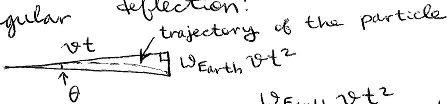
$\sin \theta \approx \theta = \frac{\omega_{\text{Earth}} v t^2}{v t} = \omega_{\text{Earth}} t$ , as expected
