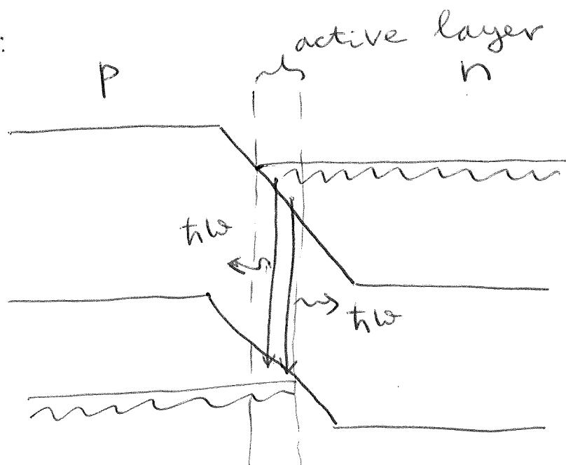
Note that photon emission is due to interband transitions and that the system is out of equilibrium ( $e^-$ 's are continuously injected on the right, recombining with holes in the active layer). The basic design of an LED is the same, but the LED operates below the lasing threshold, and no coherent amplification occurs. Finally, bandgap engineering is used to modulate the frequency of the emitted light, both in LEDs & lasers. 19.
