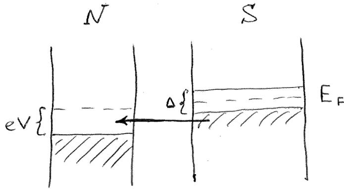
Its sign is reversed but the magnitude is independent of the sign of  $V$ , so the junction is electrically symmetric.
