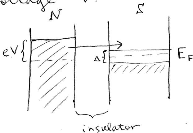
As is clear from the diagram,  $\bar{e}$  tunneling will occur once  $eV > \frac{\Delta}{2}$  ( $E_F$  is in the middle of  $\Delta$ )
