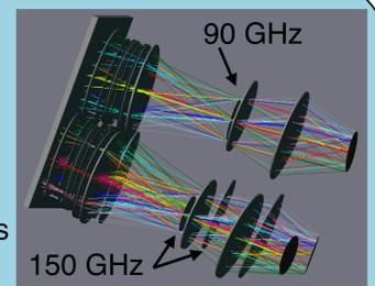
Fig. 3 - Optical path ray trace.
