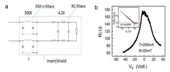
Figure C-1. a) Schematic circuit configuration for measuring the Josephson effect in graphene. b) Gate dependence of normal state resistance at T = 200mK. The superconductivity of the leads was suppressed with a small magnetic field. Inset: mean free path calculated from the transport data. The arrow indicates the onset of the puddle regime.
