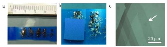
Figure A-1. Making exfoliated graphene. a) HOPG graphite flakes are deposited on Scotch tape shown with cm ruler. b) A Si/SiO<sub>2</sub> substrate is pressed onto flakes on the tape. c) Optical micrograph of graphene deposited on SiO<sub>2</sub> showing flakes with various number of layers. A large flake of single layer graphene, corresponding to the faintest contrast, is indicated by the arrow. Image credits: A. Luican-Mayer.
