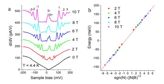
Figure B-5. Landau level spectroscopy of graphene. a) Evolution of Lnadau levels with field at 4.4 K and indicated values of field. b) LL energies plotted against the reduced parameter  $(NB)^{1/2}$  collapse onto a straight line indicating square-root dependence on level index and field. Symbols represent the peak positions obtained from (a) and the solid line is a fit to Eq.(9).
