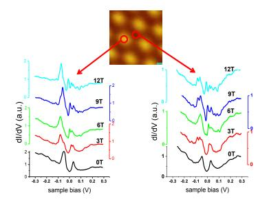
Figure B-18 Field dependence of STS for a twist angle of 1.79°. LLs ride on the van Hove singularities. The STS show strong spatial dependence across the Moiré pattern. The positions where the spectra were taken (indicated by arrows) correspond to a bright spot (left panel) and dark spot (right panel). The vertical scales in the right panels is magnified compared to the left panels to compensate for the lower signal intensity in the dark spots.
