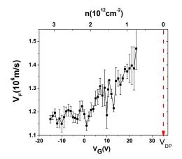
Figure B-22. Evolution of measured Fermi velocity with carriers density shows the velocity enhancement upon approaching the Dirac point. The Fermi velocity for each doping is obtained from LL spectroscopy at 12 T. The position of the Dirac point at 35V is indicated by the arrow (A.Luican,
