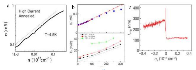
Figure C-7. a)Conductivity of suspended graphene shows  $n^{1/2}$  dependence in near-ballistic suspended graphene devices. b) Temperature dependence of minimum conductivity of suspended graphene (top) and effective Fermi energy fluctuation for suspended and non-suspended graphene (bottom). c) Mean free path in suspended graphene. On the hole side it's value is ~L/2, where L is the distance between leads.
