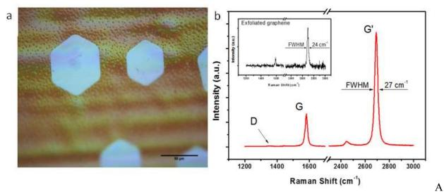
Chemical vapor deposition (CVD) on metallic substrates.
