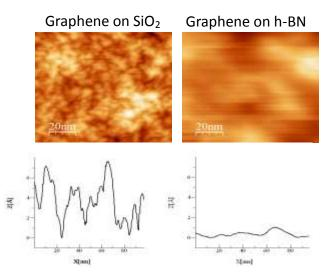
Figure B-1. STM topography of graphene on SiO<sub>2</sub> (left) and on h-BN (right). The bottom panels comparing the height variations for the two substrates show more than one order of magnitude decrease in corrugation on h-BN compared to  $SiO_2$ . (A. Luican. *et al.* 2011 unpublished). h-BN crystals were grown by K. Watanabe and T. Taniguchi
