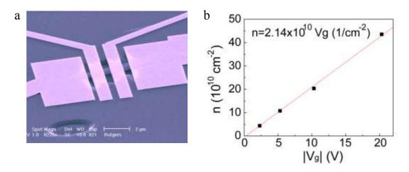
Figure C-5. a) false-color SEM image of a SG device. B) relation between gate voltage and induced carrier density obtained from magnetotransport measurements.
