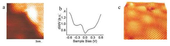
Figure B-2. STM/STS on graphene on Ru(0001) and Cu(111). a) Atomic-resolution image showing graphene overlayer across a step edge on the Ru substrate. b) Differential conductance spectrum of graphene layer on Ru substrate. Adapted from Pan et al, Adv. Mat. 21 (2009) 2777. c) Atomic resolution STM topography image of graphene on Cu showing the Moire pattern and the honeycomb structure. Adapted from Gao et al Nano Letters, 10 (2010) 3512.
