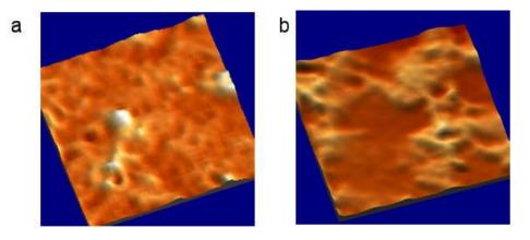
Figure B-21. DOS maps of localized and extended states in the LL regime. a) When the Fermi energy is placed in the gap between the N=0 and N=1 LLs the electronic wavefunction is localized on impurity states (bright spots in the figure). b) When the Fermi energy is within the N=1 LL the wavefunction is extended. Image credits: A. Luican-Mayer.
