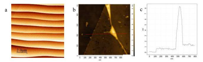
Figure A-3. a) AFM image of epitaxial graphene grown on SiC shows micron size terraces . (K.V. Emtsev *et al.* Nature Materials 8 (2009) 203). b) AFM scan (NT-MDT Integra prime) of single layer graphene flake on an h-BN substrate. c)The height profile shows a 0.7nm step between the substrate and the flake surface. The bubble under the flake is 7nm at its peak height. Image credits: B. Kim NT-MDT.
