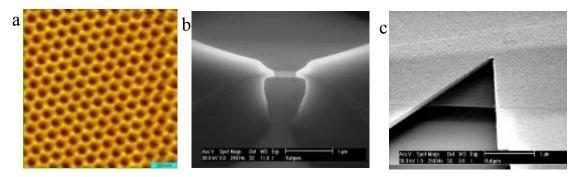
Figure A-4. STM and SEM on graphene. a) Atomic resolution STM of graphene on a graphite substrate. (b,c) SEM images on suspended graphene (FEI Sirion equipped with JC Nabity Lithography Systems). b)Suspended graphene flake supported on LOR polymer. Scale bar 1µm. Image credits: J. Meyerson. c) Suspended graphene flake (central area) held in place by Au/Ti support. Scale bar 1µm. Image credits A. Luican-Mayer.
