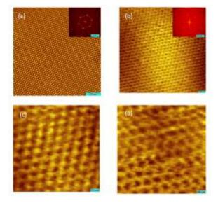
Figure B-13. Moiré pattern corresponding to a twist angle of 1.79° obtained by STM topography on a graphite surface. a) Large area image showing the super-lattice. Scale bar: 50nm. b) High resolution image showing the atomic lattice. Scale bar: 500pm. c) Zoom into a bright spot in panel *a*. Scale bar: 200pm. d) Zoom into a dark spot in panel *a*. Scale bar: 200pm. Insets: Fourier transforms of the main images.
