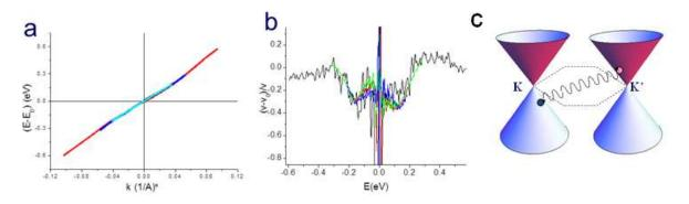
Figure B-9. a) Energy-momentum dispersion of graphene obtained from the data in Fig. B-8 as described in the text. b) Energy dependent Fermi velocity obtained by differentiating the dispersion in a. c) Schematic diagram of inter-valley scattering mediated by the A<sub>1</sub>' phonon.
