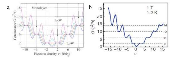
Figure C-11. a) Theoretical predictions for the two terminal conductance in the QH regime for rectangular channels with different aspect ratios [197]. b. Measured two terminal conductance in a suspended graphene device with W/L>1.
