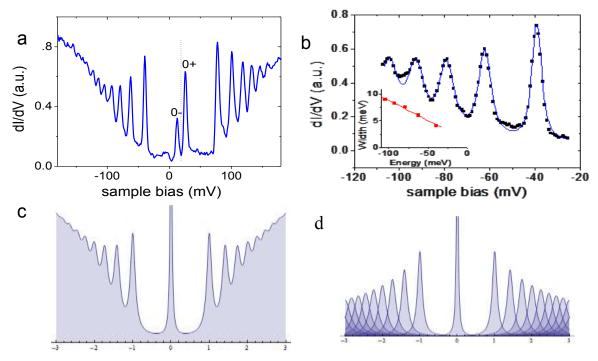
Figure B-6. Quasiparticle lifetime in graphene. a) Landau level spectrum at 4.4K and 4T. (ac modulation 2mV, setpoint 53pA at 300mV). b) High resolution spectrum on the hole side (symbols) together with a fit with sequence of Lorentzian peaks (solid line). The inset represents the energy dependence of the peak widths. c) Simulated overall density of states including the energy dependence of the linewidth. d) Individual peaks used to obtain the spectrum in c.
