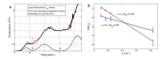
Figure C-13. a) Fit (red curve) of the two terminal resistance measured at 1.2K in 12Tesla (black curve), and extraction of longitudinal conductivity (blue curve). b) Arrhenius plot of the longitudinal conductivity obtained in (a), from which the activation energy was obtained.
