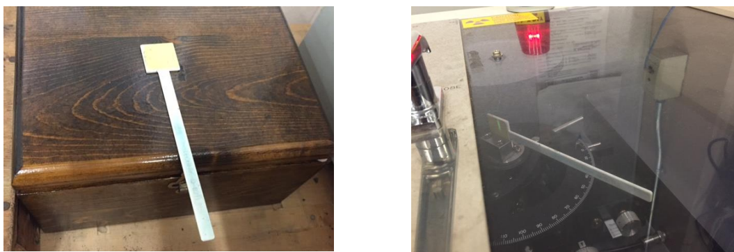
Figure 3. Fluorescent paddle. Left panel – Paddle resting on sample box. Right panel – when exposed to the X-ray beam the paddle emits green light highlighting the location of the beam.
