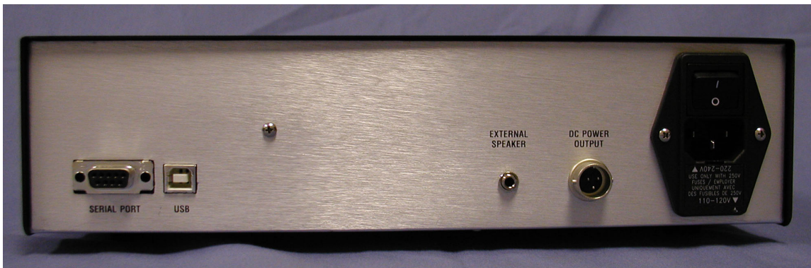
Figure 7. Rear of electronics box. The communications ports are on the left. Use only one.
