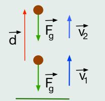
Freely falling object moving upwards:
