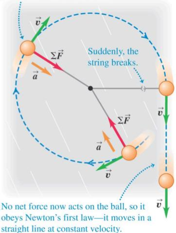
ball attached to a string in uniform circular motion on a horizontal frictionless plane
