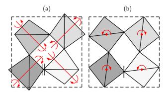
FIG. 1. (Color online) Projection on x-y plane of the (a)  $\tilde{\alpha}$  and (b)  $\tilde{\beta}$  structures, proposed as candidates for  $\alpha$  and  $\beta$  cristobalite phases, respectively. Darker shading is used to represent more distant tetrahedra so that the spiral structure of the connected tetrahedrons becomes evident; double vertical lines indicate that the adjoining tetrahedra are actually disconnected because they are separated in the z direction.
