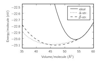
FIG. 2. Ground-state energy per formula unit (eV) vs volume per formula unit (Å<sup>3</sup>) for  $\tilde{\alpha}$ ,  $\tilde{\beta}$ , and cubic cristobalite structures of SiO<sub>2</sub>.
