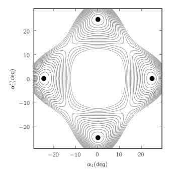
FIG. 6. Energy as a function of rotation angles  $\phi_{\alpha_1}$  and  $\phi_{\alpha'_1}$ , corresponding to rotations  $\tilde{\alpha}_1$  and  $\tilde{\alpha}'_1$  shown in Fig. 3. The origin corresponds to "ideal" cristobalite. The four minima (filled circles) correspond to the  $\tilde{\alpha}'_1$  structure (top and bottom) and to the  $\tilde{\alpha}_1$  structure (left and right). The energy difference separating contours is 3 meV per SiO<sub>2</sub> formula unit.
