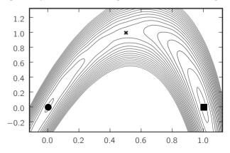
FIG. 4. Energy in plane defined by the  $\tilde{\alpha}$  structure (filled circle),  $\tilde{\beta}$  structure (filled square), and saddle point (cross). Coordinates are chosen such that these structures occur at (0,0), (1,0), and (0.5,1), respectively. The energy difference separating contours is 3 meV per SiO<sub>2</sub> formula unit.
