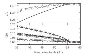
FIG. 8. Structural parameters of the  $\tilde{\alpha}$  structure vs volume per formula unit. Top panel: c/a ratio. Bottom panel: absolute values of deviations of internal parameters u(Si) (squares), x(O) (triangles), y(O) (crosses), and z(O) (circles) from ideal-cubic values. Symbols represent first-principles calculations; lines are fits to an ideal rigid-unit geometry.
