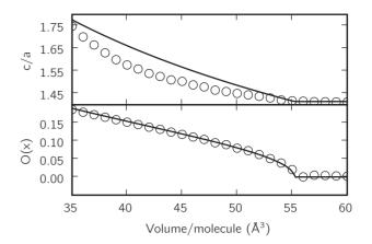
FIG. 9. Structural parameters of the  $\tilde{\beta}$  structure vs volume per formula unit. Top panel: c/a ratio. Bottom panel: x(O). Symbols represent first-principles calculations; lines are fits to an ideal rigid-unit geometry.
