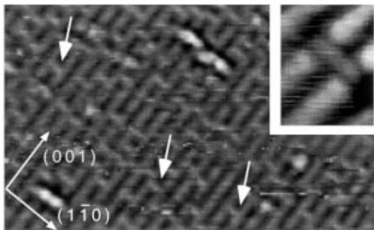
FIG. 3. STM image of a slightly oxygen-deficient  $\text{TiO}_2(110)$  surface,  $190 \times 120 \text{ \AA}^2$ . The arrows point to the features assigned as single oxygen vacancies, one of which is enlarged in the inset. Sample bias +1.2 V, tunneling current 0.5 nA.
