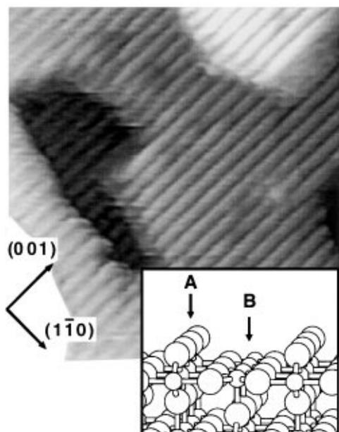
FIG. 1. STM image of a stoichiometric  $1 \times 1$   $\text{TiO}_2(110)$  surface,  $140 \times 140 \text{ \AA}^2$ . Sample bias +1.6 V, tunneling current 0.38 nA. The inset shows a ball-and-stick model of the unrelaxed  $1 \times 1$   $\text{TiO}_2(110)$  surface. Rows of bridging oxygen atoms are labeled "A," rows of fivefold coordinated titaniums "B."
