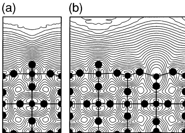
FIG. 2. Contour plots of [001]-averaged charge densities associated with electron states within 2 eV of the conduction band minimum for (a) the relaxed stoichiometric  $1 \times 1$  surface and (b) the relaxed oxygen-deficient  $2 \times 1$  surface. Contour levels correspond to a geometric progression of charge density, with a factor of 0.56 separating neighboring contours. The "noise" in the topmost contours is an artifact of the periodically repeated slab geometry.
