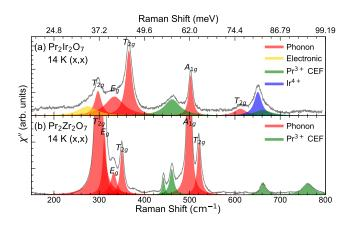
FIG. 1. Raman scattering spectra of (a)  $Pr_2Ir_2O_7$  and (b)  $Pr_2Zr_2O_7$  at 14 K in parallel polarization configuration.
