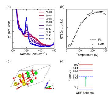
FIG. 4. (a) Temperature dependence of Raman scattering spectra of  $Pr_2Zr_2O_7$  in the region of  $A_{1g} \rightarrow E_g$  crystal electric field transitions in (x, y) channel. (b) Temperature dependence of spectral weight  $I(T) = \int_{430 \text{ cm}^{-1}}^{330 \text{ cm}^{-1}} \chi''(\omega) d\omega$ . (c) Atomic displacement of  $T_{2g}^{(2)}$  phonon mode. (d) Crystal field scheme of  $Pr^{3+}$  ions in  $Pr_2Zr_2O_7$  crystal environment.
