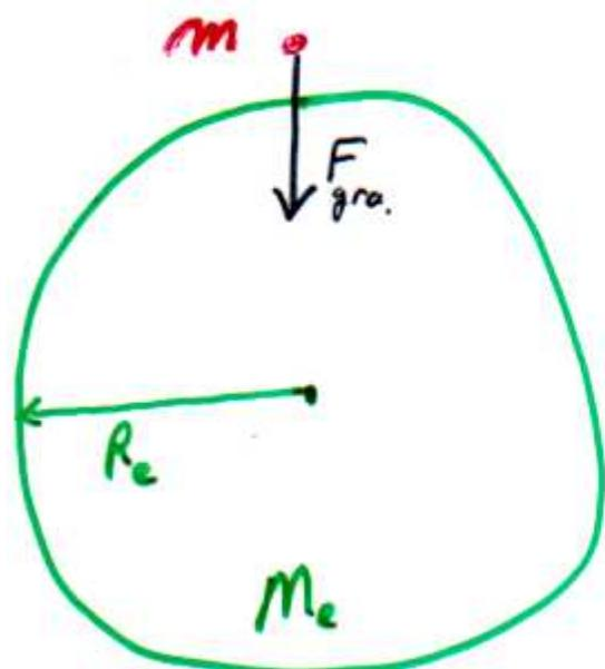
$$F_{\text{grav}} = \frac{G M_e m}{R_e^2} \quad \text{N. U. L. G.}$$
