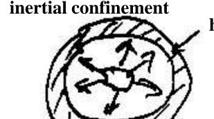
high Z material resists expansion by virtue of the inertia of its mass (tamper)
