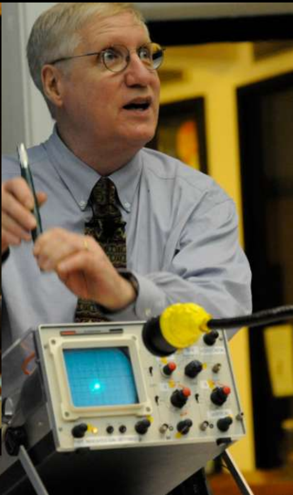
Magnetic field deflects electron beam to the side.
