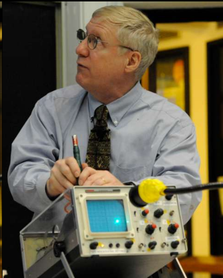
Magnetic field deflects electron beam to the side.
