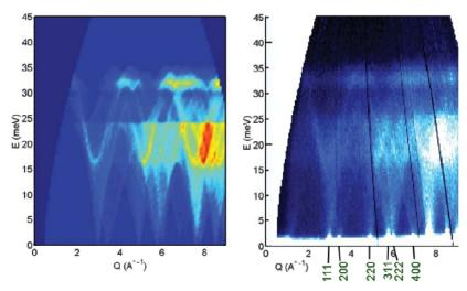
Comparison between computed (left) and measured (right) inelastic scattering of neutrons by phonons in polycrystalline fcc Ni-Fe.
