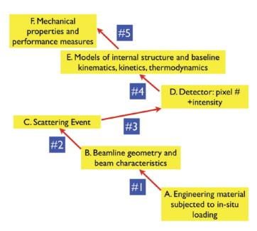
Schematic depicting the aspects (A-F) of a high-energy x-ray diffraction experiment designed to quantify the internal microstructure and micromechanical response of an engineering alloy.
