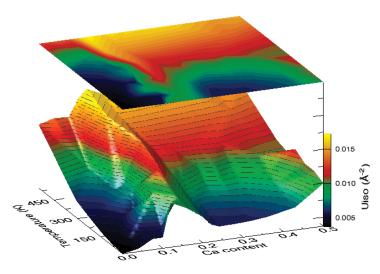
This figure shows the power of high throughput diffraction studies coupled with advanced computation. Local oxygen displacements in La<sub>1-x</sub>Ca<sub>x</sub>MnO<sub>3</sub> are presented as a function of x and T, showing fluctuations associated with a structural phase transition (the ridge around x=0.15), the disappearance of polarons (the blue valley at low temperature and x~0.3), and a competition between phases of similar energy (the small valley at around x=0.5 and 260 K).
