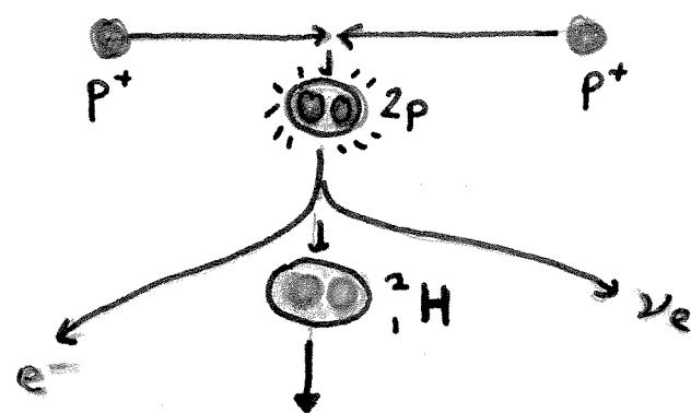
$$\begin{aligned} \text{Coulomb Energy barrier} &= U = \frac{e^2}{4\pi\epsilon_0 r} = \frac{(1.6 \times 10^{-19} \text{ C})^2 \times (9 \times 10^9 \text{ Nm}^2/\text{C}^2)}{2 \times 10^{-15} \text{ m}} \\ &\approx 1.2 \times 10^{-13} \text{ J} \\ &= \underline{\underline{0.7 \text{ MeV}}} \end{aligned}$$
