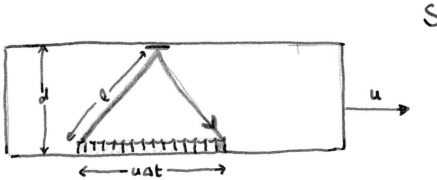
We'll see the clock ticks every  $\Delta t$  seconds, and during this time, the train moves forwards a distance  $u\Delta t$ . The distance travelled by the light is  $2l$ , where
