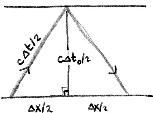
$$\left(\frac{c\Delta t}{2}\right)^2 = \left(\frac{c\Delta t_0}{2}\right)^2 + \left(\frac{\Delta x}{2}\right)^2$$
