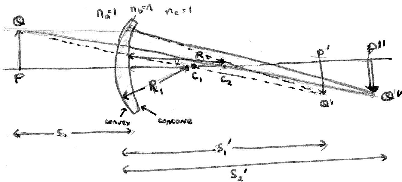
The light refracting off the second surface is focussed at a distance  $s'_1$  to the right of the surface, and behaves as an object at position  $s_2 = -s'_1$  for the second surface.
