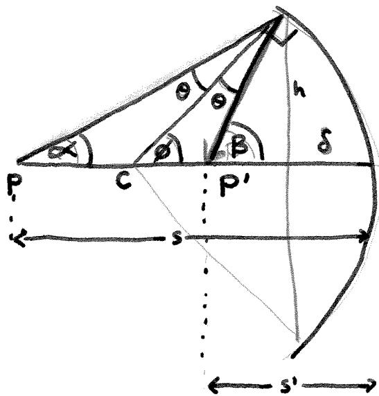
$$\begin{aligned} \alpha + \theta &= \phi \\ \phi + \theta &= \beta \end{aligned} \quad \left. \begin{array}{l} \text{exterior } \angle \\ = \text{sum of opp} \\ \text{interior } \angle s. \end{array} \right\}$$
