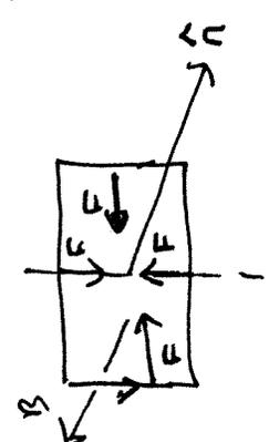
All the forces on the wire produce no torque
