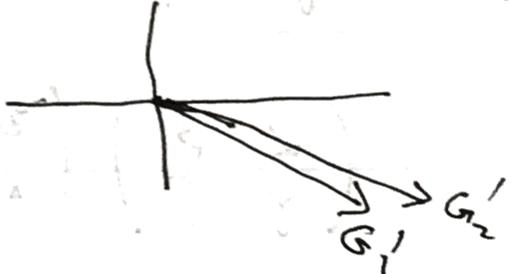
$$(dG)_{\text{space}} = (dG)_{\text{body}} + (dG)_{\text{rot}}$$
