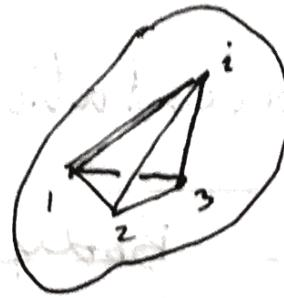
Distance between any pair of particles fixed
