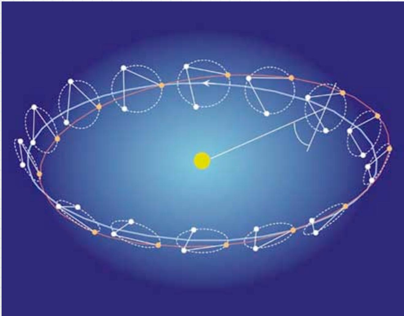
The LISA constellation follows the earth in a tumbling orbit. This constant change in orientation allows good determination of the GW source position and orientation, thus breaking the degeneracy and allowing a unique determination of the luminosity distance.
