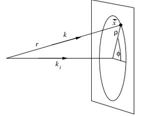
The contribution for very large values of  $z$  will come from  $\rho \sim \sqrt{z}$  so the angle goes to zero,  $\vec{k} = \vec{k}_i$ ,  $kr - \vec{k}_i \cdot \vec{x} = k(r - z) = k(\sqrt{z^2 + \rho^2} - z) \approx k\rho^2/2z$ , so<sup>2</sup>
