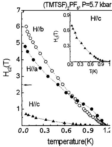
Figure 1. Resistively determined critical field along the principle axes for (TMTSF)<sub>2</sub>PF<sub>6</sub>, P=5.7 kbar. Insert is expansion of c axis data. All curves are well above the calculated Ginzburg-Landau values. Horizontal arrow indicates the Pauli limiting field for singlet superconductivity.
