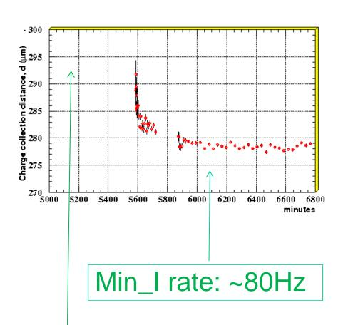
Pulse height drops with rate about 5% in 300 minutes
