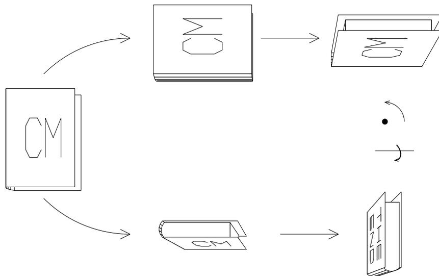
Figure 4.1: The results of applying the two rotations  $H$  and  $V$  to a book depends on which is done first. Thus rotations do not commute. Here we are looking down at a book which is originally lying face up on a table.  $V$  is a rotation about the vertical  $z$ -axis, and  $H$  is a rotation about a fixed axis pointing to the right, each through  $90^\circ$ .
