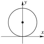
For an object which has some thickness, with non-zero  $z$  components, the perpendicular axis theorem becomes an inequality,  $I_{zz} \leq I_{xx} + I_{yy}$ .
