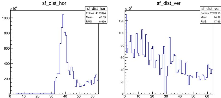
FIG. 3. Hits as a function of fiber number for the SciFi array at the IFP. Here the 96 fibers are put into the final 32 channels of the horizontal histogram and the 64 channels of the vertical histogram. Data were taken with positive beam polarity at 158 MeV/c, using a random pulser trigger. Due to the construction of the array and the configuration at the IFP, the array was offset vertically so that the beam went through the array close to one end.
