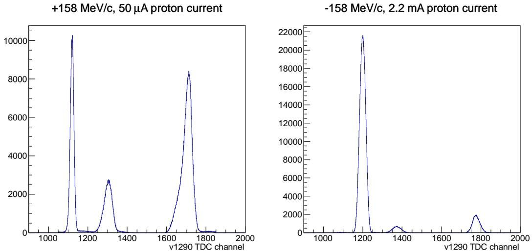
(a) Run 180, 158 MeV/c, 50  $\mu$ A proton beam current. (b) Run 211, -158 MeV/c, 2.2 mA proton beam current.
