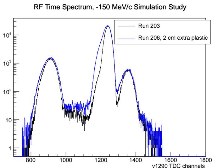
FIG. 4. RF time spectra for run 203 (black) and run 206 (blue). Conditions were the same, except for an extra 2 cm of plastic added into the IFP region for run 206.
