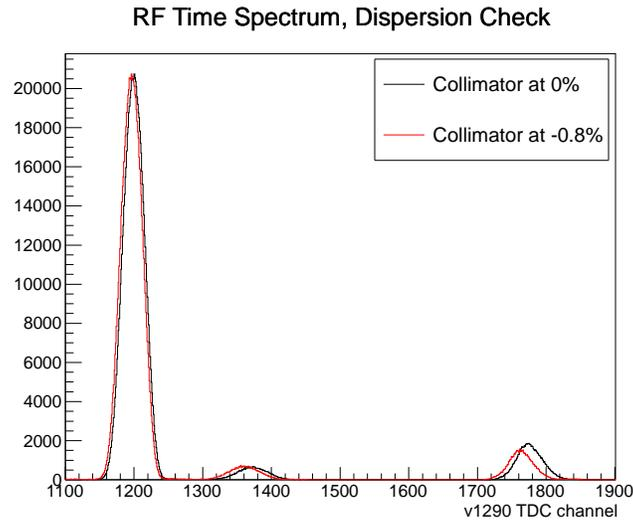
FIG. 2. RF times at the target for some runs checking dispersion with a collimator at  $\approx 0\%$  (black spectrum) and  $\approx -0.8\%$  (red spectrum). Beam conditions were 2.2 mA of primary protons, with front jaws set to 300. Small shifts in the  $\mu$  peak at the right near channel 1350 and the  $\pi$  peak near channel 1800 can be seen, while the electron peak position is essentially constant.
