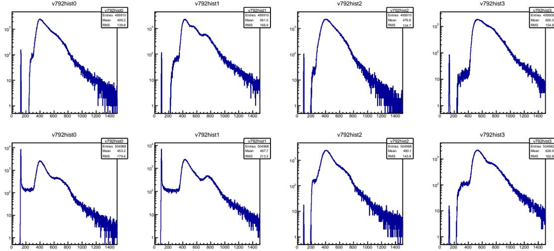
FIG. 5. QDC spectrum for trigger scintillator phototubes from runs 223 (top) and 232 (bottom) at  $-158$  MeV/c. The spectra are for (from left) SBL, SBR, SAL, and SAR. See text for details.
