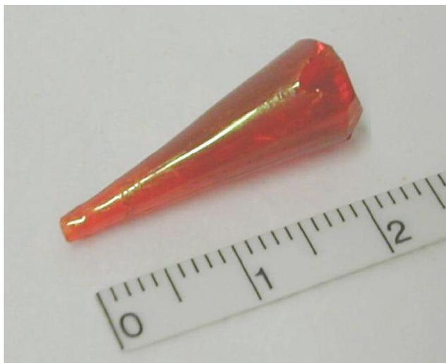
**FIGURE 2.1.4** A tetracene crystal grown by the vapor-Bridgman technique and used for the time-of-flight studies. (From Niemax, J. et al., *Appl. Phys. Lett.*, 86, 122105, 2005.)
