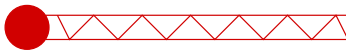
FIGURE 12. In a superconductor, a magnetic monopole (small ball) is the source of a flux tube. As a result, its energy grows linearly with the size of the system.
