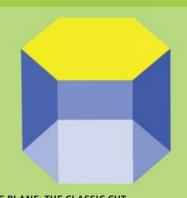
C-PLANE: THE CLASSIC CUT Though commonly used for blue lasers, a *c*-plane substrate has drawbacks, such as inducing electric fields that conspire to ke
