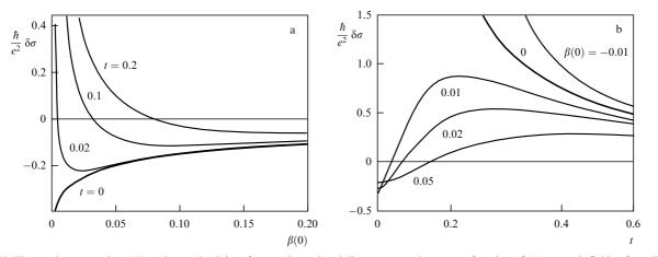
Figure 10. Fluctuation correction (48) to the conductivity of a two-dimensional dirty superconductor as a function of (a) magnetic field at four different temperatures, and (b) temperature at five different strengths of the magnetic field [59]. Thick curves are the separatrices of both families of the curves.
