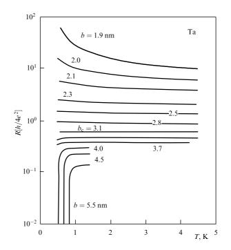
Figure 38. Temperature dependences of the resistance of amorphous ultrathin Ta films of different thicknesses [145]. The superconducting transition temperature decreases with thickness b and becomes zero at b = 3.1 nm.
