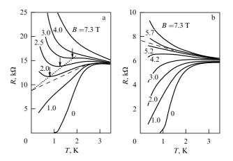
**Figure 25.** Families of temperature dependences of resistance of two amorphous In-O films 200 Å thick in different magnetic fields. The separatrices of both families are shown by dashed lines. In figure (a), the critical value  $R_c$  (intercept of the separatrix with the ordinate axis) is determined by the extrapolation of the positions of the minima marked by the arrows in the R(T) curves (dotted line) [105, 106].
