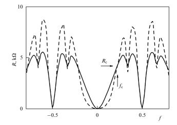
**Figure 45.** Resistance of a Josephson junction array with a normal resistance  $R_{\Box} = 10.5 \text{ k}\Omega$  and parameter x = 0.9 as a function of frustration *f* at a temperature of 180 mK (solid curve) and 80 mK (dashed curve) [166]. The arrows indicate the critical values of the resistance ( $R_c$ ) and frustration ( $f_c$ ) determined as the coordinates of the point of intersection of the isotherms.
