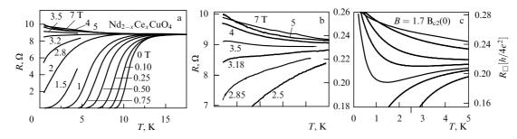
**Figure 39.** (a) Temperature dependences of the resistance of an epitaxial  $Nd_{2-x}Ce_xCuO_4$  film 1000 Å thick [148]. (b) Part of Fig. 39a on an enlarged scale; the negative derivative of the resistance with respect to temperature is seen  $(\partial R/\partial T < 0)$  in the fields exceeding the critical one, as is the intersection of the curves in the fields of 5 and 7 T. (c) R(T) functions calculated with formulas (48) and (109) [148].
