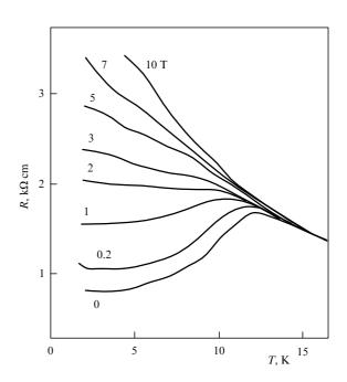
Figure 36. Temperature dependence of the longitudinal magnetoresistance  $R_{ab}$  of a two-dimensional organic superconductor  $\kappa$ -(BEDT-TTF)2Cu[N(CN)2]Cl at a small pressure in a magnetic field perpendicular to the two-dimensional layers [140].
