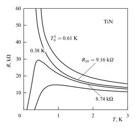
**Figure 32.** Superconductor–insulator transition in a zero magnetic field in a family of TiN films. Film resistances at T = 10 K are given for the two middle curves (these can be assumed to be a control parameter); for the two upper curves, the activation energies  $T_0^1$  are indicated [116].
