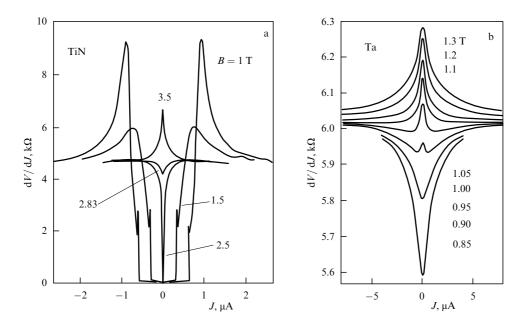
Figure 42. Differential resistance  $\partial V/\partial J$  of films near the superconductor-insulator transition in various magnetic fields as a function of a dc current through the film. The measurement temperature was less than 0.1 K. (a) TiN films 5 nm thick with a superconducting transition temperature  $T_c \approx 1$  K [152]; signs of hysteresis phenomena are seen in the curves at B = 1 and 1.5 T. (b) Ta films 5 nm thick with  $T_c \approx 0.67$  K [154].
