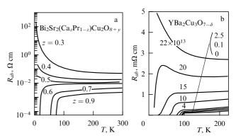
**Figure 33.** (a) Temperature dependences of the resistance of  $Bi_2Sr_2(Ca_zPr_{1-z})Cu_2O_{8+y}$  samples at various Ca concentrations (indicated alongside the curves) [118]. (b) Temperature dependences of the resistance of a YBCO film after a stepped change in the dose of irradiation with Ne<sup>+</sup> ions [122]. The doses are indicated near the curves as the number of ions per cm<sup>2</sup>.
