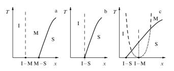
**Figure 2.** Variants of the phase diagram with transitions between three different states of the electron system: insulator (I), normal metal (M), and superconductor (S). The quantum transitions are shown by dots lying on the abscissa; the thermodynamic transitions, by solid curves; the cross-overs and the boundaries of the critical region, by dashed lines, and the virtual boundaries in figure (c), by dotted lines.
