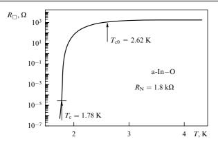
**Figure 6.** Temperature  $T_{c0}$  at which an equilibrium concentration of Cooper pairs appears, and the temperature  $T_c$  of the BKT transition in an In-O film 100 Å thick [30].  $R_{\Box}$  is the resistance per square (resistivity of a two-dimensional system).
