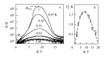
**Figure 28.** (a) Family of five R(B) isotherms of an amorphous In – O film with thicknesses of 200–300 Å in state 1 (see text) in a perpendicular magnetic field [109]. (b) Variation of the activation energy  $T_0^1$  with strengthening magnetic field, obtained from an analysis of isotherms; on both edges of the interval of magnetic fields, the accuracy of determining  $T_0^1$  decreases because of the closeness to the phase transition points [109].
