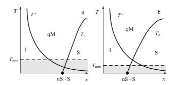
**Figure 37.** Two variants of the phase diagram for two-dimensional systems. Curve  $T^*(x)$  is plotted with formula (108); the dashed straight line  $T = T_{min}$  specifies the temperature range  $T > T_{min}$  in which all realistic experiments are performed; qM denotes quasimetal, and nS, nonsuperconductor (analogous diagrams for three-dimensional systems were given in Fig. 2).
