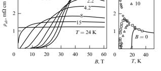
Figure 35. (a) Longitudinal magnetoresistance  $\rho_{ab}$  of an LSCO single crystal, measured in a pulsed magnetic field at various temperatures [134]. (b) Temperature dependences  $\rho_{ab}(T)$  in a field B = 0 (solid curve) and B = 10, 20, and 60 T (data points) [134].
