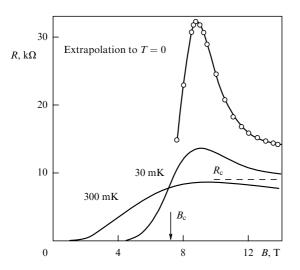
**Figure 29.** Magnetoresistance of an amorphous In–O film 200 Å thick whose representative point lies relatively deep in the superconducting region [107]. The upper curve is drawn through points (shown by circles) obtained by the extrapolation of the experimental values of R(T) at various *B* to T = 0 using formula (104).
