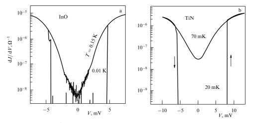
**Figure 43.** Differential conductivity dJ/dV of an InO film in a magnetic field of 2 T at two temperatures (indicated alongside the curves) [155]. (b) Differential conductivity dJ/dV of a TiN film in a magnetic field of 0.9 T [116]. The difference in the voltages at which the upward and downward jumps occur indicates the existence of a hysteresis.
