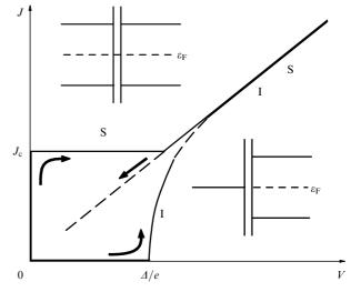
**Figure 41.** Superconductor–superconductor (in the upper part of the figure) and normal metal–superconductor (in the right-hand part of the figure) tunnel junctions, and a schematic of their zero-temperature current–voltage characteristics.
