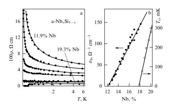
**Figure 1.** (a) Temperature dependences of resistivity  $\rho(T)$  of films of the amorphous Nb<sub>x</sub>Si<sub>1-x</sub> alloy at various concentrations of Nb [6]. (b) Dependences of the superconducting transition temperature  $T_c$  and of the extrapolated value of the low-temperature conductivity  $\sigma_0 = \lim \sigma(T \to 0)$  on the Nb concentration in films of the amorphous Nb<sub>x</sub>Si<sub>1-x</sub> alloy [6].
