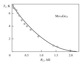
**Figure 7.** Suppression of superconductivity by a disorder in amorphous  $Mo_{79}Ge_{21}$  films [40]. Circles correspond to experimental data taken from Refs [41, 42], and the solid curve was constructed from formula (15).
