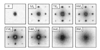
**Figure 47.** Diffraction of a testing laser beam in a system of ultracold <sup>87</sup>Rb atoms depending on the amplitude of the periodic potential created by standing laser waves; the wave amplitude is indicated in the upper left-hand corner of each pattern [171].
