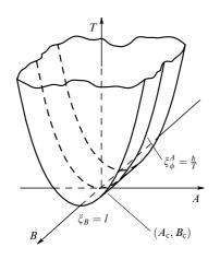
Figure 17. Critical vicinity of a saddle point in a flow diagram for twoparametric scaling.
