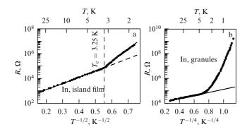
**Figure 4.** (a) Temperature dependence of the resistance of an In island film exhibiting a significant *increase* in the resistance at temperatures less than the temperature of the superconducting transition in indium granules. (b) The same for a granular film consisting of In granules separated by insulating oxide interlayers [22].
