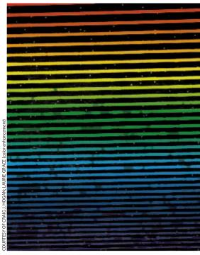
KECK TELESCOPE (*right*) on Mauna Kea, Hawaii, gathered light from a distant quasar and concentrated it on the photodetector of a highresolution spectroscope. The resulting bands of color (*above*) are marked by dark lines where intervening gases have absorbed light of specific wavelengths. Analysis of the characteristic line patterns for hydrogen gas can reveal the presence of the heavy isotope of the element deuterium.
