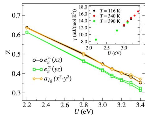
FIG. 5. (Color online) Renormalization constants  $Z_\alpha = [1 - \partial \text{Re } \Sigma_\alpha(\omega) / \partial \omega]^{-1}$  of the different orbitals in the  $R$  phase as a function of  $U$ . Inset: electronic specific heat,  $\gamma = \sum_\alpha \rho_\alpha(0) / Z_\alpha$ , calculated at different temperature and values of  $U$ .
