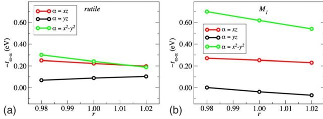
FIG. 3. (Color online) The intradimer V-V hoppings corresponding to the  $t_{2g}$  orbitals shown in Fig. 2 as a function of strain. The left (right) panel shows the parameters in the rutile ( $M_1$ ) phase. The direction of strain is depicted in Fig. 1.
