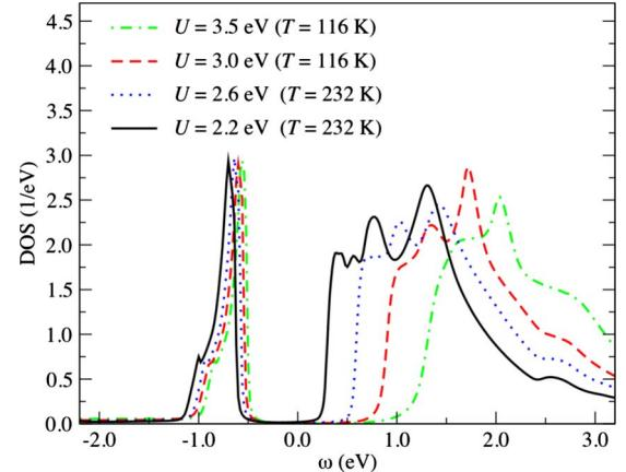
FIG. 4. (Color online) The variation of the  $t_{2g}$  density of states of the  $M_1$  phase as a function of the applied Coulomb repulsion parameter,  $U$ . Note the high sensitivity of the gap on  $U$ .
