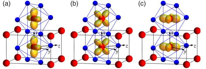
FIG. 2. (Color online) The sketch of vanadium  $t_{2g}$  orbitals [(a)  $d_{x^2-y^2}$ , (b)  $d_{xz}$ , (c)  $d_{yz}$ ] together with the applied coordinate system and the V-V pairs considered in the rutile phase calculations. Large (red) spheres: V atoms, small (blue) spheres: O atoms.
