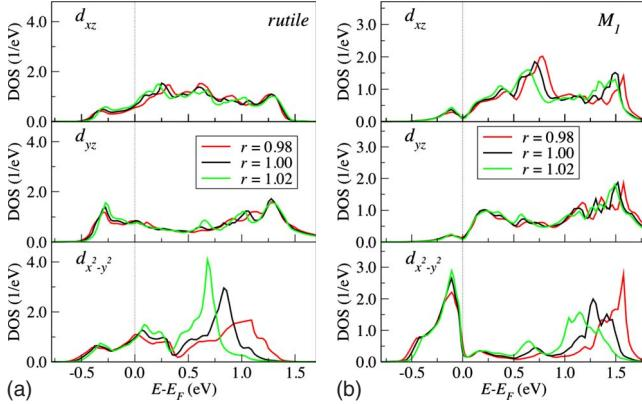
FIG. 6. (Color online) LDA partial DOS of the  $t_{2g}$  states of a V atom in the rutile (left) and  $M_1$  (right) phases in the proximity of the Fermi energy with different  $r$  ratios:  $r=0.98$  (dotted, red), 1.00 (full, black), and 1.02 (dashed, green). Note the large splitting of the  $d_{x^2-y^2}$  peaks and the barely changed DOS at the Fermi level.
