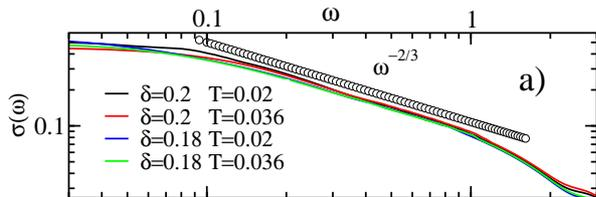
FIG. 31: (Color online) The optical conductivity  $\sigma(\omega)$  of the t-J model is proportional to  $\omega^{-2/3}$  in the intermediate frequency region for optimally doped system.
