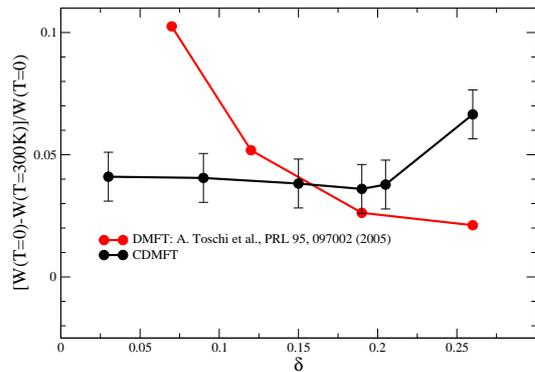
FIG. 33: (Color online) Difference between the low temperature and 300K optical spectral weight integrated up to  $\Lambda = 6t$ . The cluster data are computed within EDCA and the single site DMFT results are reproduced from Ref. 123). The error bars are due to extrapolation of spectral weight to zero temperature from finite temperature results ( $T_{min} \sim 0.5T_c$ ).
