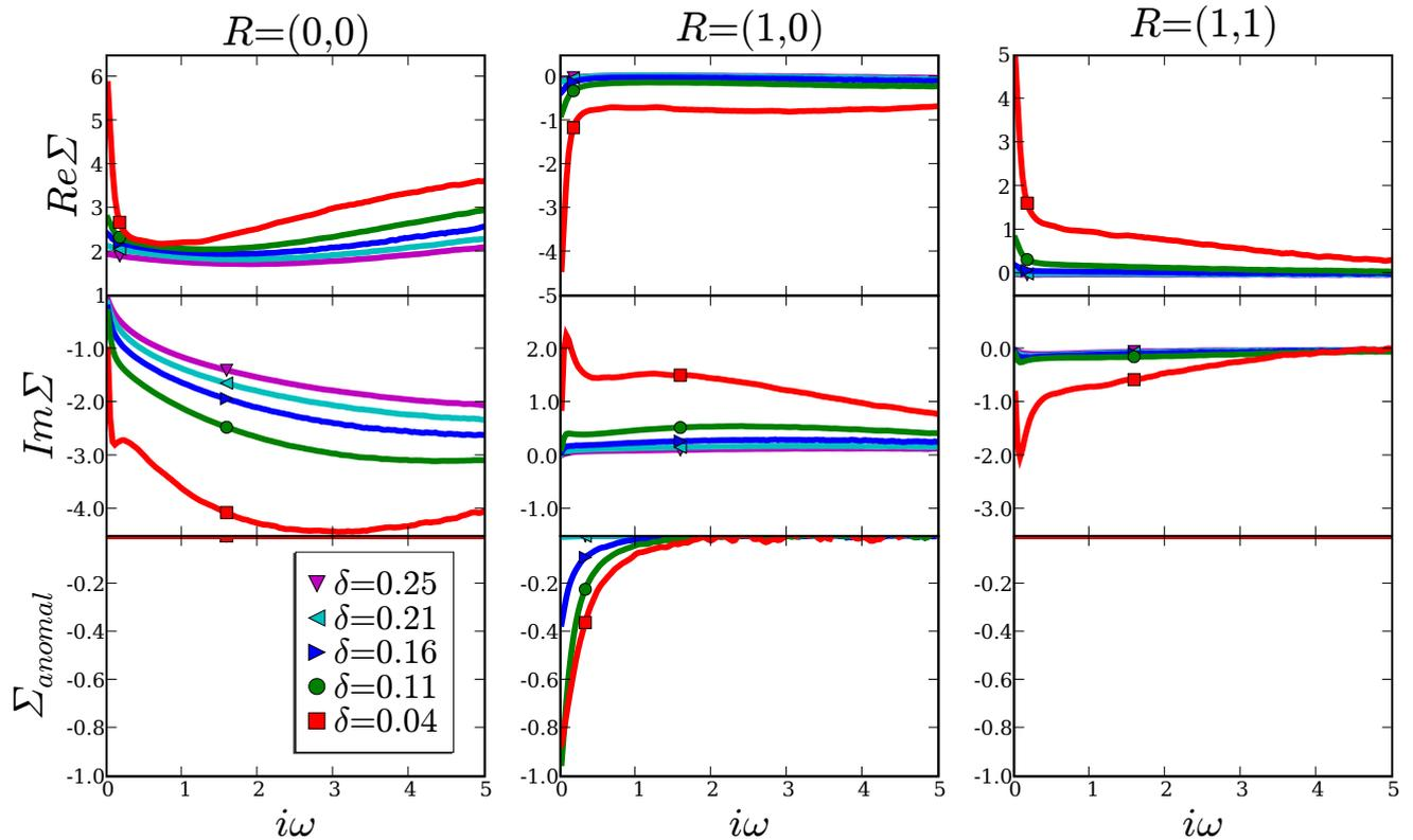
FIG. 10: (Color online) The on-site and short range self-energy of the Hubbard model in the superconducting state at  $T = 0.005t$ . The on-site self-energy is the largest and its imaginary part vanishes for all finite dopings. The reason is that the pole in the  $(\pi, \pi)$  self-energy is now at zero doping. The non-local components of the self-energy vanish rather rapidly with doping.
