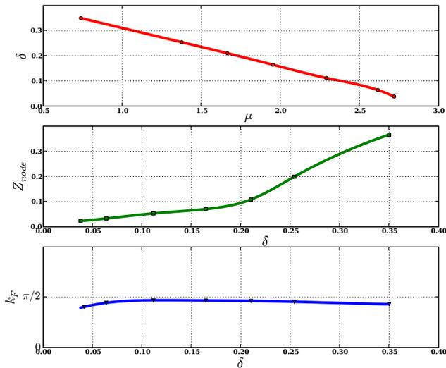
FIG. 26: (Color online) upper panel: doping versus the chemical potential for the Hubbard model at  $T = 0.005t$ . It shows linear dependence and downturn at small doping. This could point to divergence of the compressibility zero doping. middle panel: the nodal quasiparticle residue  $Z$  versus doping. It is slowly increasing in the underdoped and optimally doped system and increases rather rapidly in the overdoped system. lower panel: fermi momentum along the nodal direction versus doping.
