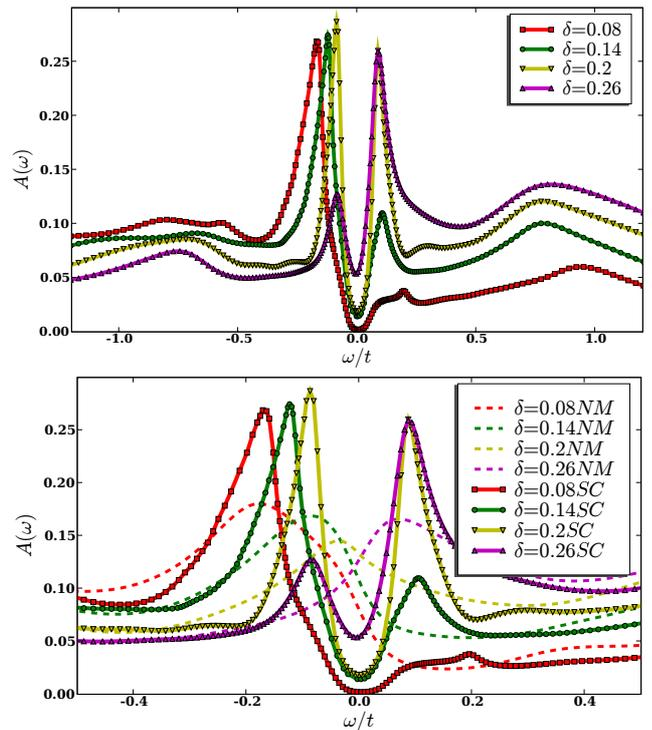
FIG. 25: (Color online) Tunneling density of states (local spectral function) in EDCA obtained with NCA at constant  $T = 0.025t$ . The lower panel is a blow up of the low energy regions. The dotted lines show the normal state spectral function for the same doping and temperature.
