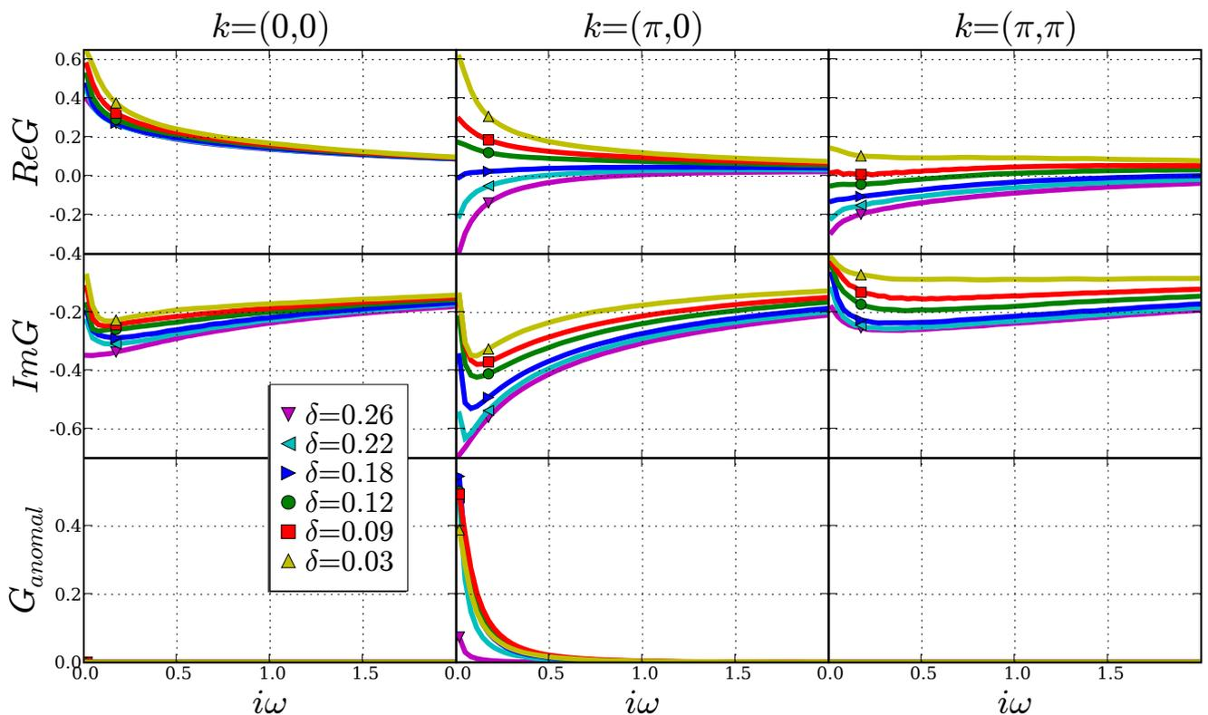
FIG. 7: (Color online) C-DMFT cluster Green's functions of the  $t$ -J model at  $T = 0.005t$  in the superconducting state obtained by CTQMC. Superconducting gap opens in particular in  $(\pi,0)$  orbital. Particle-hole symmetry of this orbital is again evident from the real part of the Green's function being close to zero around optimal doping (blue curve with triangles pointing right).
