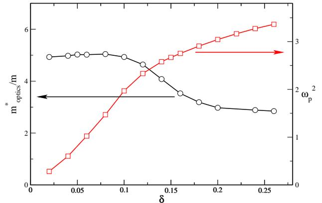
FIG. 30: (Color online) effective mass and plasma frequency as a function of doping. Obtained from optical conductivity of Fig. 28.
