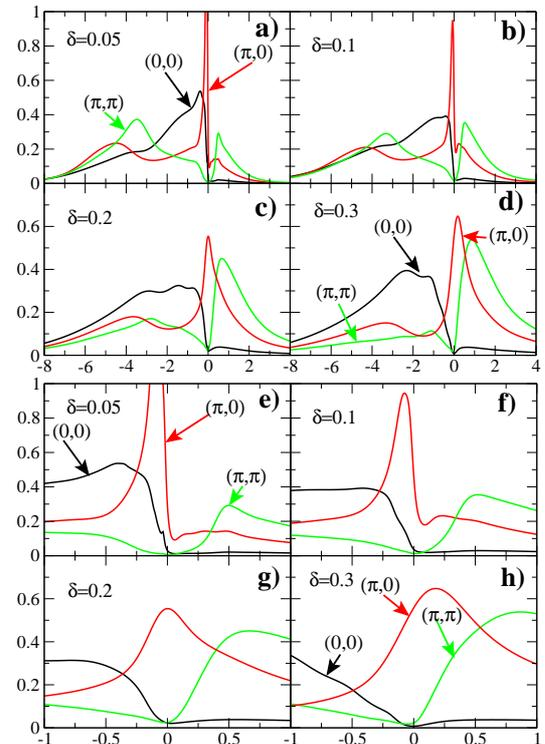
FIG. 13: (Color online) Evolution of the EC-DMFT cluster spectral functions of the t-J model with doping in normal state at  $T = 0.025t \sim T_c$  using NCA as an impurity solver. The upper panel shows the spectra in the interval between  $[-8t, 4t]$  where Hubbard band is clearly observed. The lower panel shows the region near the Fermi level.
