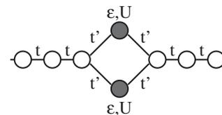
FIG. 1. Schematic representation of the model for a parallel double quantum dot coupled to two semi-infinite tight-binding chains with equal hopping constants. The Fermi level is fixed at zero energy.
