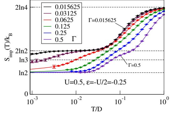
FIG. 2 (color online). Comparison of the impurity entropy curves at the particle-hole symmetric point. Lines: NRG; circles: QMC results (with error bars). Energy unit is the half-bandwidth  $D = 1$ .
