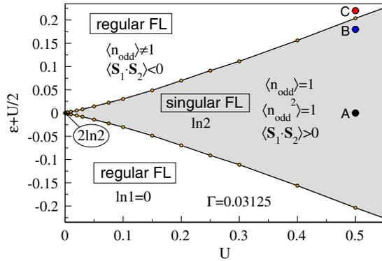
FIG. 4 (color online). Phase diagram in the  $(\epsilon, U)$  plane obtained by using the NRG. The entropy curve at point A is shown in Fig. 2, while those at points B and C are compared in Fig. 3.
