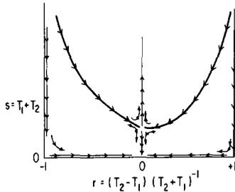
FIG. 3. Renormalization group flows for the anisotropic  $SO(N) \times SO(N-1)$  model in  $2 + \epsilon$  dimensions (see Part II, Section 3.3). The broad lines are phase boundaries (critical surfaces).  $N = 3$ ,  $\epsilon > 0$ .
